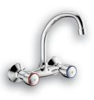
Two hole, wall type with swivel outlet. 1/2" BSP male connection ends. Chrome plated
